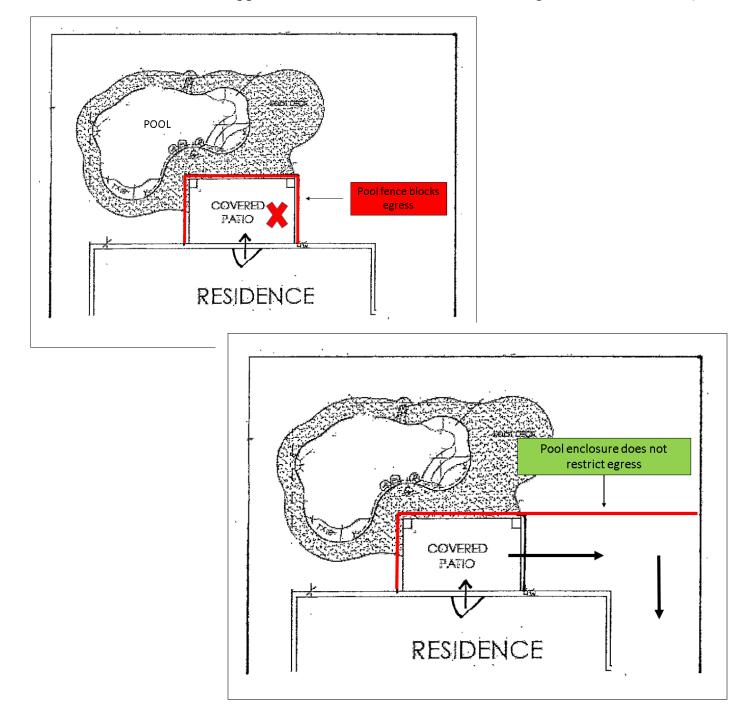
A door from the home does not open into the pool enclosure or is permanently locked or barricaded with no key accessible to a child.
